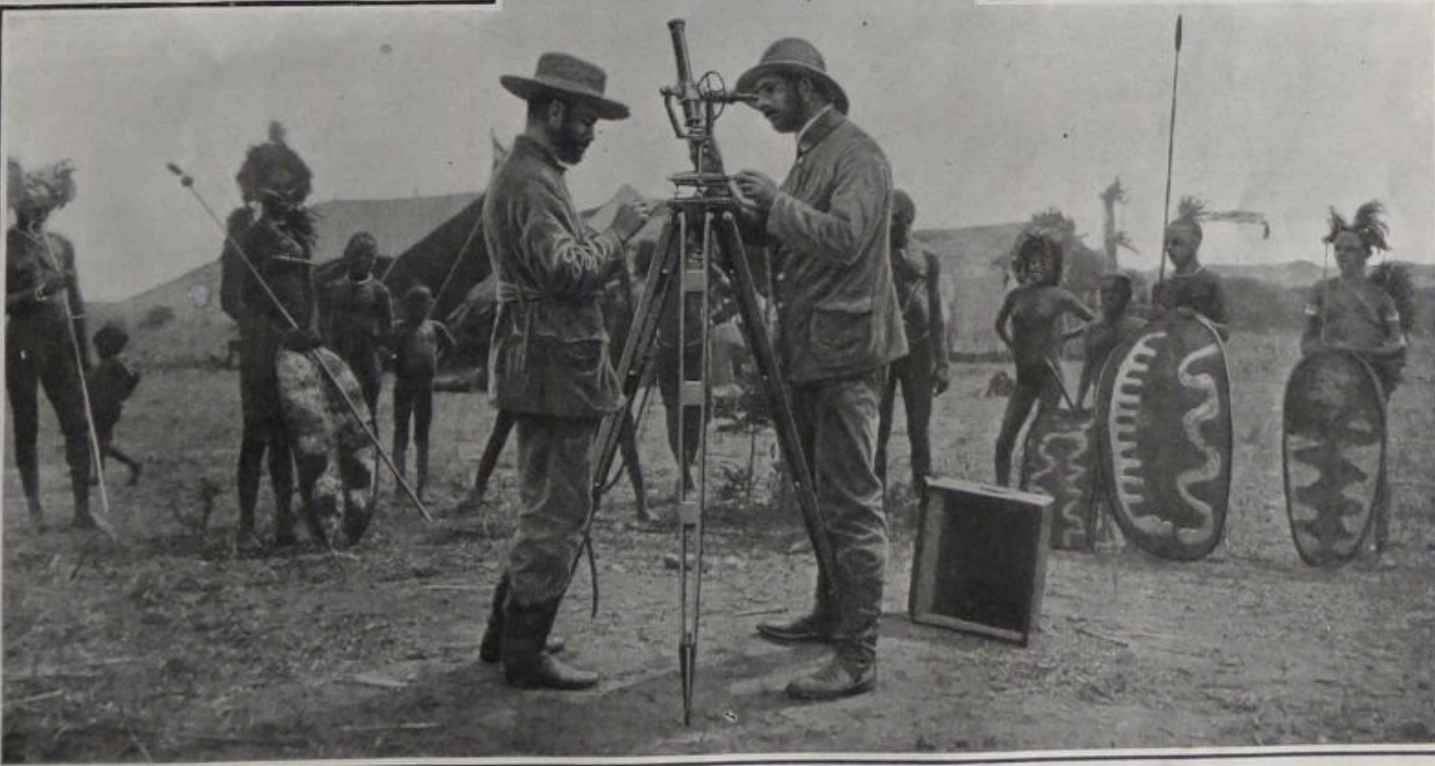
Noting the course of pilot balloons with special theodolites. The pilot balloons are liberated to ascertain the direction and velocity of the wind before the liberation of registering balloons.
