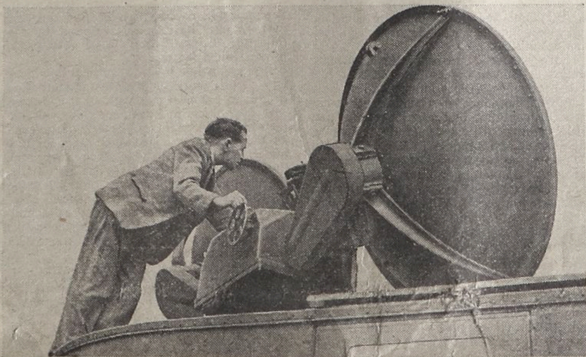
Radar aerials are seen in use at Kew Observatory to follow a radio-sonde balloon of the standard Meteorological Office type.
