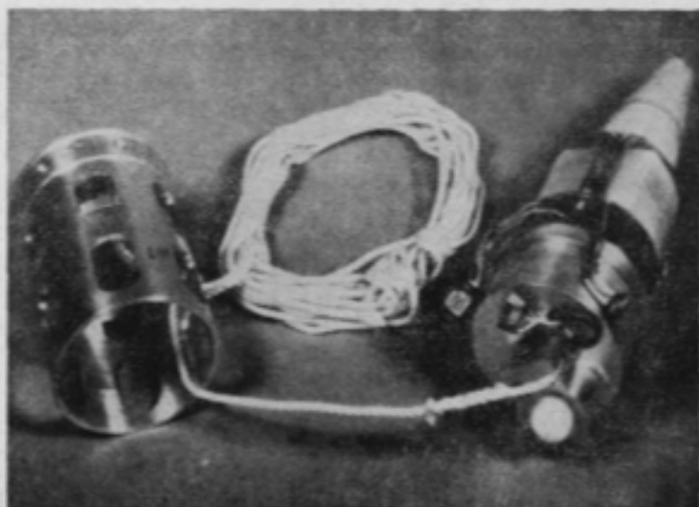
ROCKET-BORNE instrument is designed to test the deployment system for the ROCOZ ozonesonde soon to be used in a series of Arcas rocket flights.
